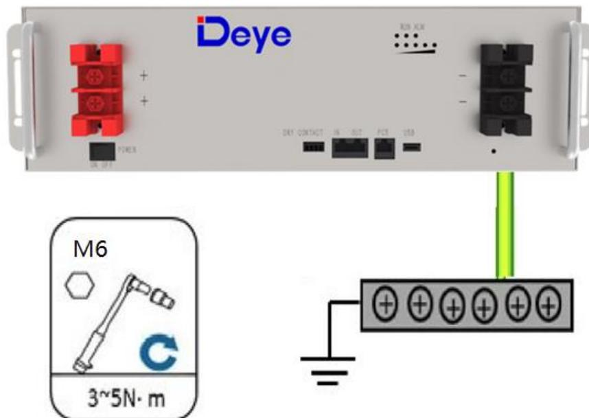
Figure 5-1: Install the Grounding Wire
