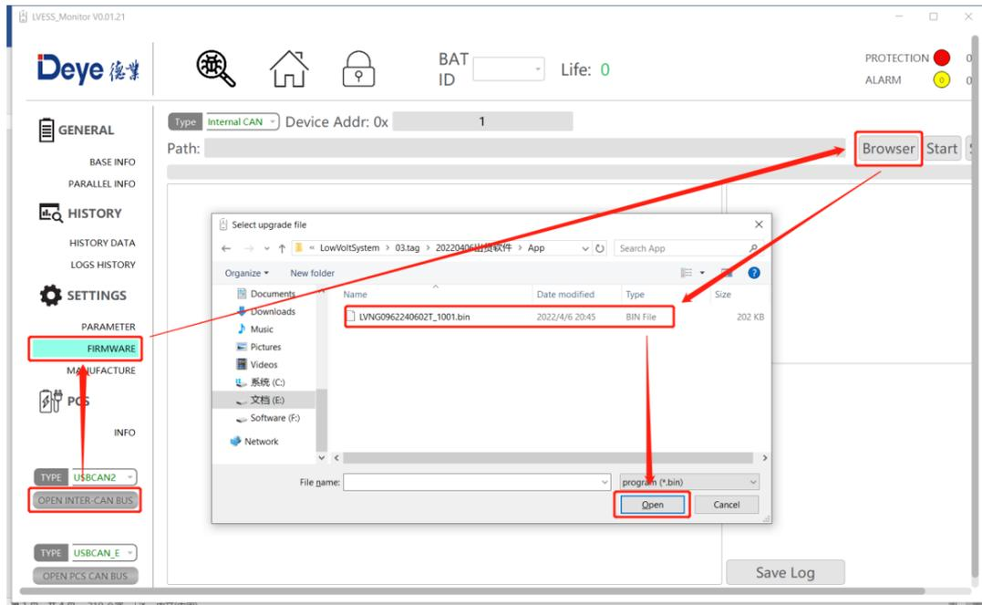
Step 2. Select the upgrade pack number, if there is "0x" in "Device Address", enter the corresponding hexadecimal number, such as upgrading Pack No. 29, enter 1D; if there is no "0x" in "Device Address", enter the corresponding decimal number No., if you upgrade Pack No. 25, enter 25.
