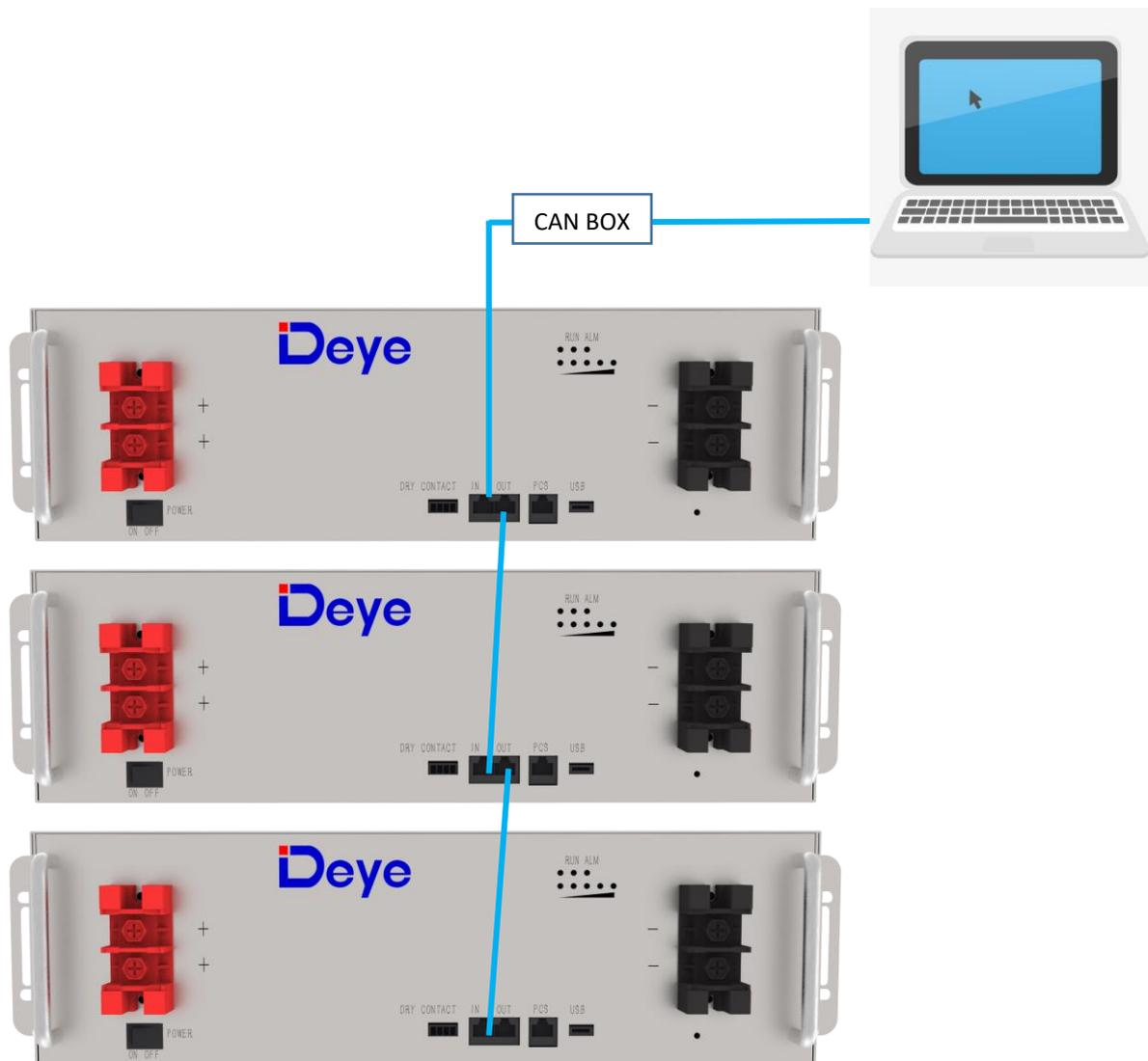
Figure 5-3: Communication Cable Connections between Battery and Computer
