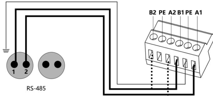
3. The inverters are connected to the ShineMaster via RS485 serial connection. Using the RS485 wired communication connection, the ShineMaster can monitor up to 64 inverters stably.
