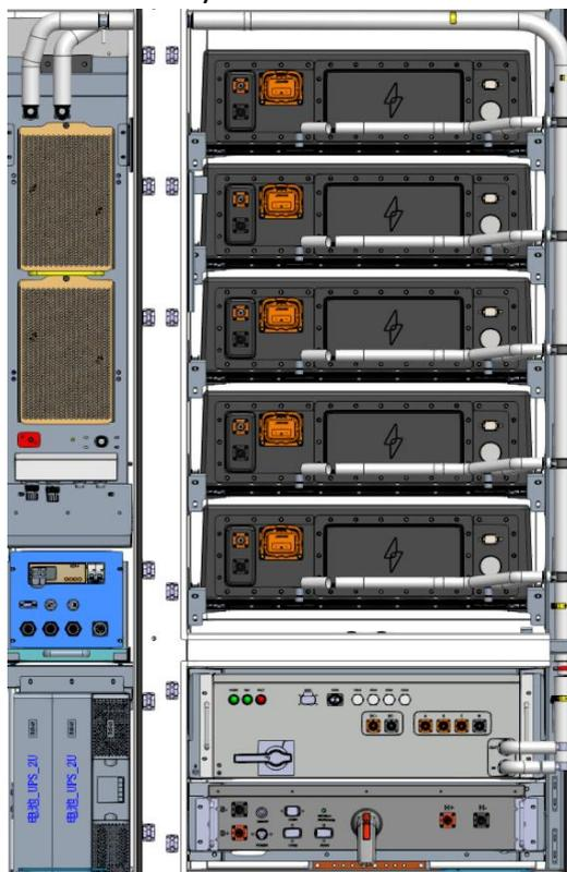
**Chart 3-12 Liquid Cooling Pipe Installation Schematic**
