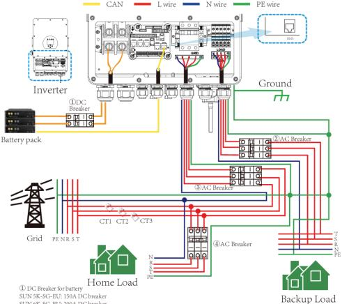
© DC Breaker for battery SUN 5K-SG-EU: 150A DC breaker SUN 6K-SG-EU: 200A DC breaker SUN 8K-SG-EU: 250A DC breaker SUN 10K-SG-EU:300A DC breaker SUN 12K-SG-EU:300A DC breaker
